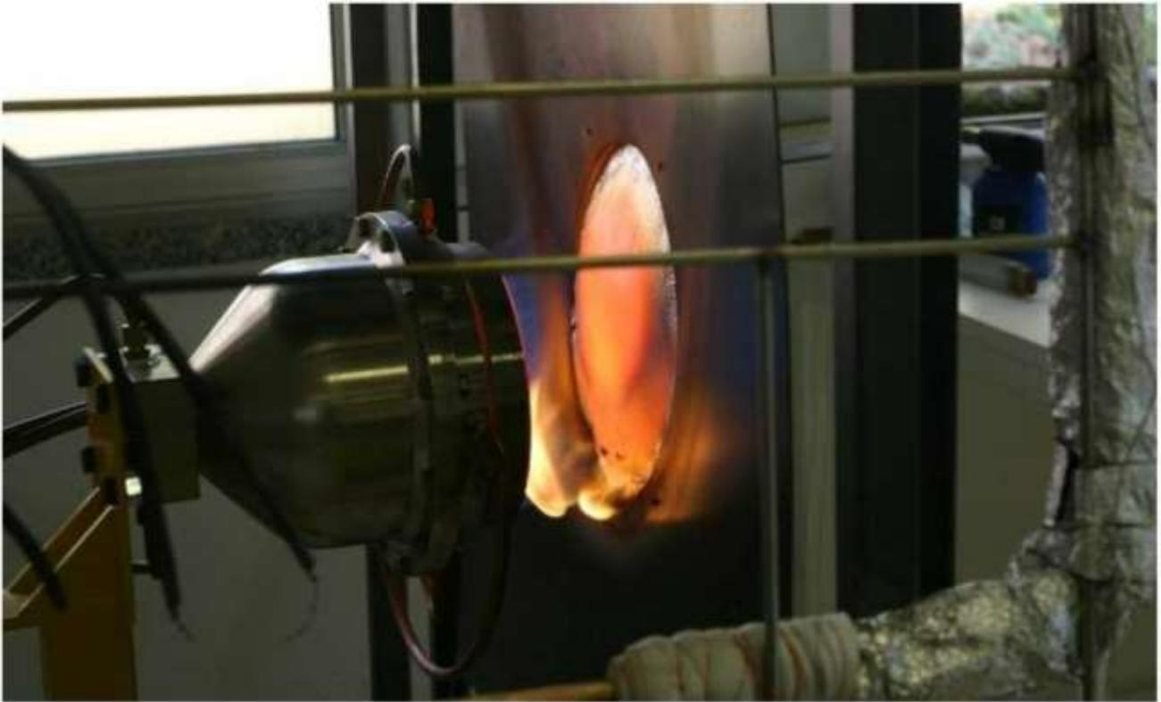
The specimen was mounted at a distance of 82 mm from the nose of the burner.
